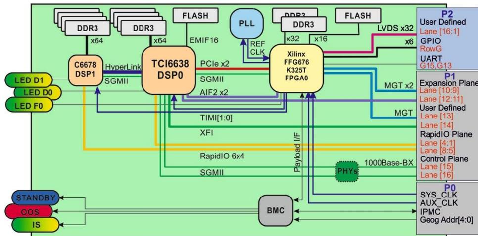
Figure 3: CommAgility VPX-D16A4 Block Diagram
